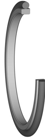
The double-action SPOR30 consists of a PTFE-bronze sealing element and an O-ring that serves as a pre-tensioning element.
